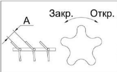
The diagram illustrates the mechanical adjustment of the grate shutter. On the left, a perspective view shows the shutter mechanism with a label 'А' pointing to the shutter blades. On the right, a top-down view shows the star-shaped opening formed by the shutter blades. Arrows labeled 'Закр.' (Closed) and 'Откр.' (Open) indicate the direction of movement for the shutter blades to adjust the opening size.
